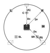
• Setting Centre Speaker If the distance of Dc is equal to or longer than the DF in the left figure, set the mode as 0ms. Otherwise, change the setting according to the table below.
